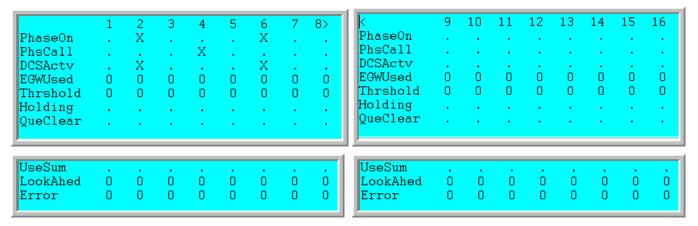
Each column's entries have the data for one phase. The screen shots above indicate that phases 2 and 6 are the D-CS controlled phases.
