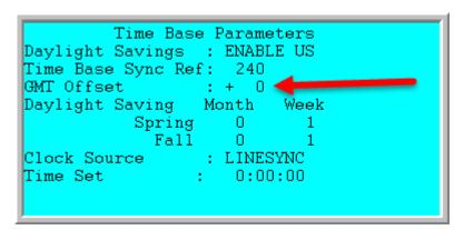
Using the Garmin external GPS, the controller will automatically resynchronize the time from the GPS unit twice per hour at approximately 13 and 43 minutes past the hour, every hour.
