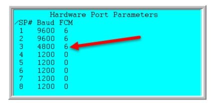
Note: Whenever the Agency modifies the hardware binding (MM->6->6) the unit has to be restarted via a physical power down/up.
