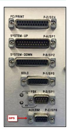
Note: Whenever the Agency modifies the hardware binding (MM->6->6) the unit has to be restarted via a physical power down/up.
