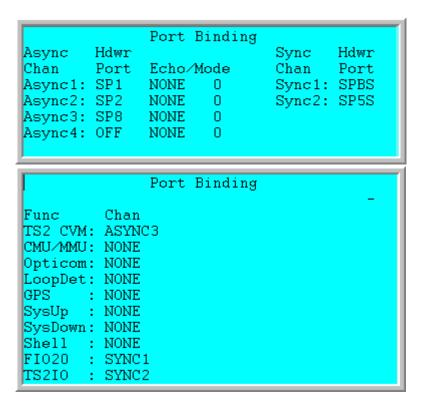
By accessing the Port Binding sub-menu at MM->6->6, the user can assign the GPS unit to interface to the bottom port of the 2070-7A (SP2 = ASYNC2) as shown on the screen shots below.
