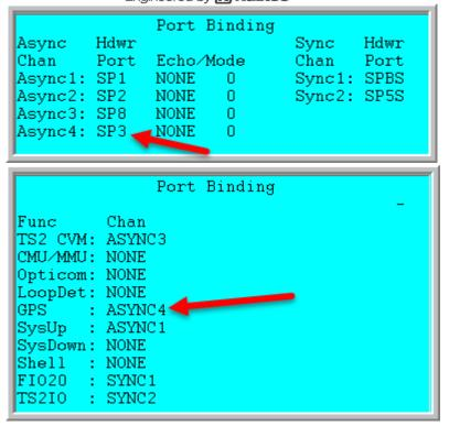
In the example above, SP3 on a 2070-7T or 2070-7G card is assigned to the GPS unit.
