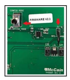
The Intelight GPS switch "S1" must be set with switch 1 in the down position and switch 2 in the up position as shown to the right. Switch 2 is set to establish the internal async connection when mounted inside the controller.
