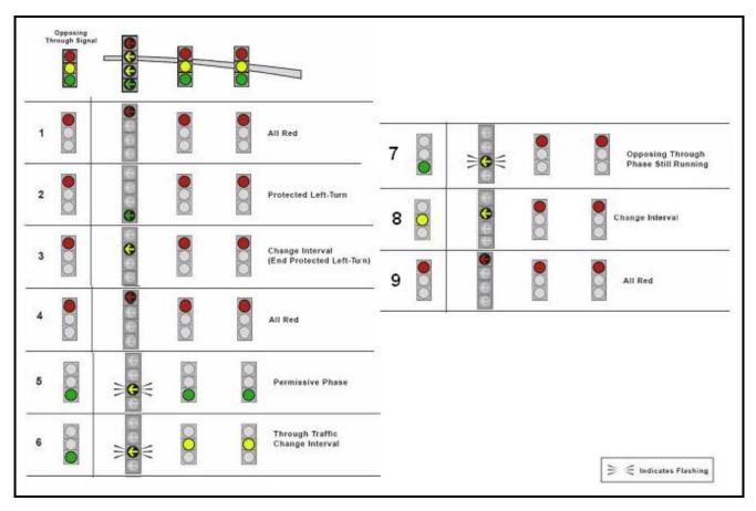
Once an agency determines how to set up their intersections, they may want to operate them in free or coordinated modes. Lead /Lag lefts are normally engineered for the best traffic flow during Free operation (fixed recalls or actuated detection). When a user operates signals in coordination they may use lead/lag phasing to improve green band efficiency. In addition, because SynchroGreen adaptive uses coordination as its basis, it could also be impacted.
