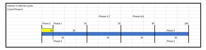
Note that Phase 2 (the Pseudo-Coordinated Phase) bridges between the last cycle and the new cycle. In fact, once the next cycle begins phase 2 only has 5 seconds of green begore it clears to run Phase 1. This could have un intended results.
