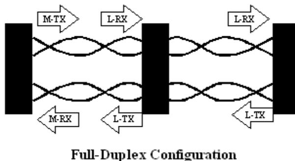
In this configuration, the master modem (the one on the farthest left), has a single pair dedicated to its transmission. The local modems (center, right) utilize the master's transmit pair only for receiving. Because the master is the only unit transmitting on this pair, it is acceptable for the unit to be constantly driving the line (**RTS/CTS** active). In fact, by constantly asserting the **RTS** signal, the turn around time that it usually
