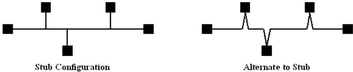
A word of caution, however. In the alternate configuration, notice that the total length of the transmission line increases by twice the sum of all the stub lengths. This needs to be considered, because controlling reflection can be accomplished, while a signal that has been completely attenuated is not recoverable.
