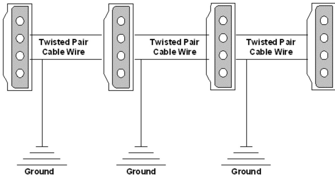
In the diagram above, the agency has decided to be consistent by grounding each cable as it exits each modem (or signal cabinet.).
