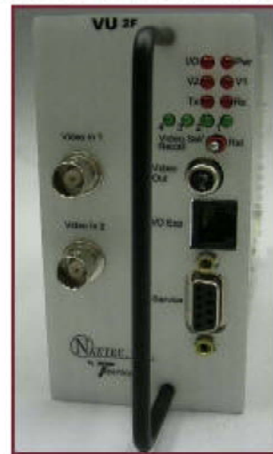
VU1 and VU2 Vehicle Presence and Data Detector
