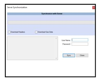
Logging into the ATMS server is required for syncing. In addition, the log-in will reflect the jurisdictional control that is set up in ATMS. Therefore, by logging-in the user's StreetSync database will only synchronize the databases that they are allowed to use. The user must provide a username and password as shown below.
