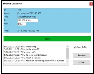
Selecting **Retrieve** will get the data from the Local event data. The Clear Buffer selection will clear the buffer in the controller after retrieving the data. Once the data is retrieved a report is generated on the overview pane which displays the data. There are four Local Event categories that can be displayed: Alarms, Patterns, Preemption and transit. Below is an Alarm data sample.
