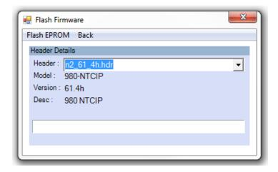
Click on the pull down menu to select the firmware header file. A list will appear, with the available Proms to download. Select the desired EPROM. Finally, Select **FlashEPROM** from the menu to begin the download. The header files must be located on the ATMS server under the directory: ...Naztec/Nazserv/Downprom.
