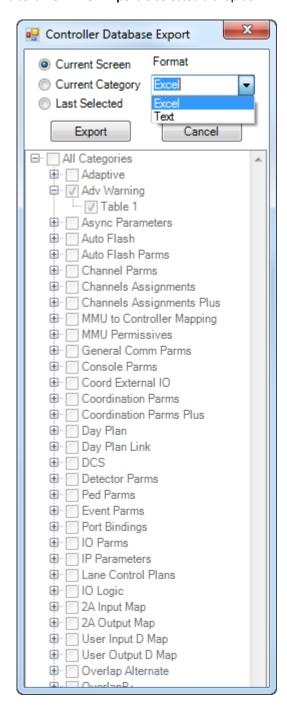
The user can select which sheets to export out via the radio buttons on the top of the screen.
