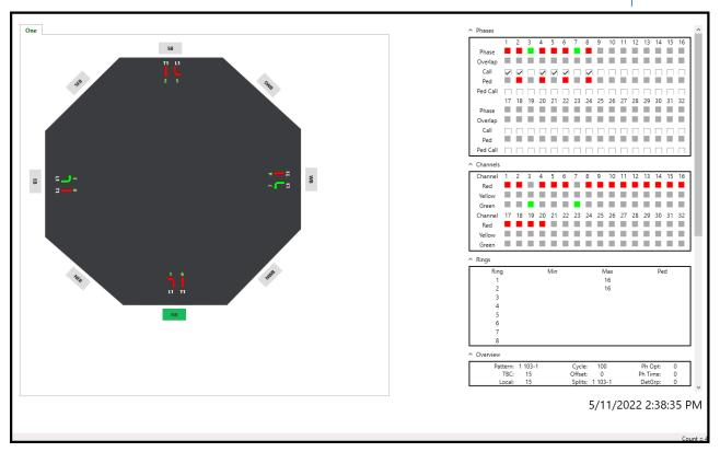
The scan screen will display Phase Red/Yellow/Green status, timing, Channel Outputs and coordination data so that the user can check the intersection from his PC while verifying field data. In addition, the user can view live alarm data as well as detection data by sliding down the bar on the right side of the screen.
