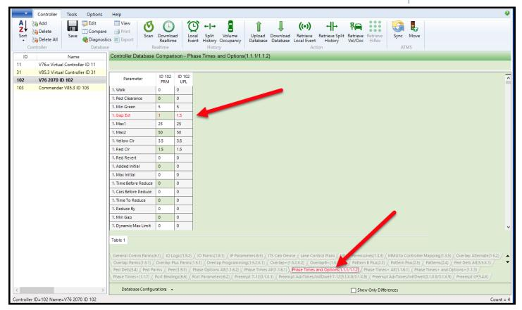
Differences are easily located and identified between the StreetSync database (PRM) and the uploaded database from the controller (UPL). Database differences are shown by color coding each database category tab and corresponding database parameter in RED. This will occur when a difference is present between the database types.
