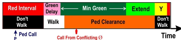
Green Delay Used to Suppress the Start of Green When a Ped Call is Serviced
