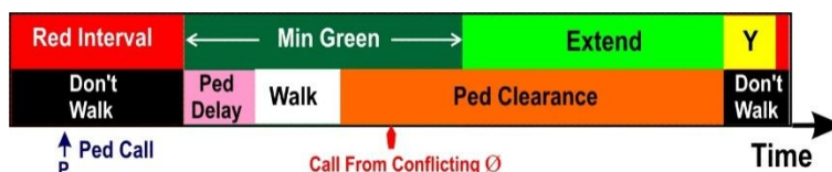
Ped Delay Used to Suppress the Start of Walk When a Ped Call is Serviced
