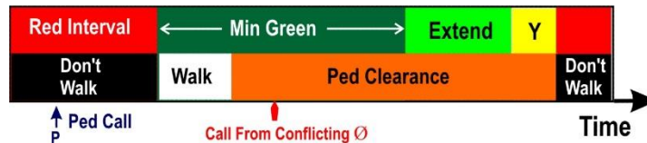
Ped Clearances Times With Vehicle Clearance if PedClr-Thru-Yellow is Enabled
